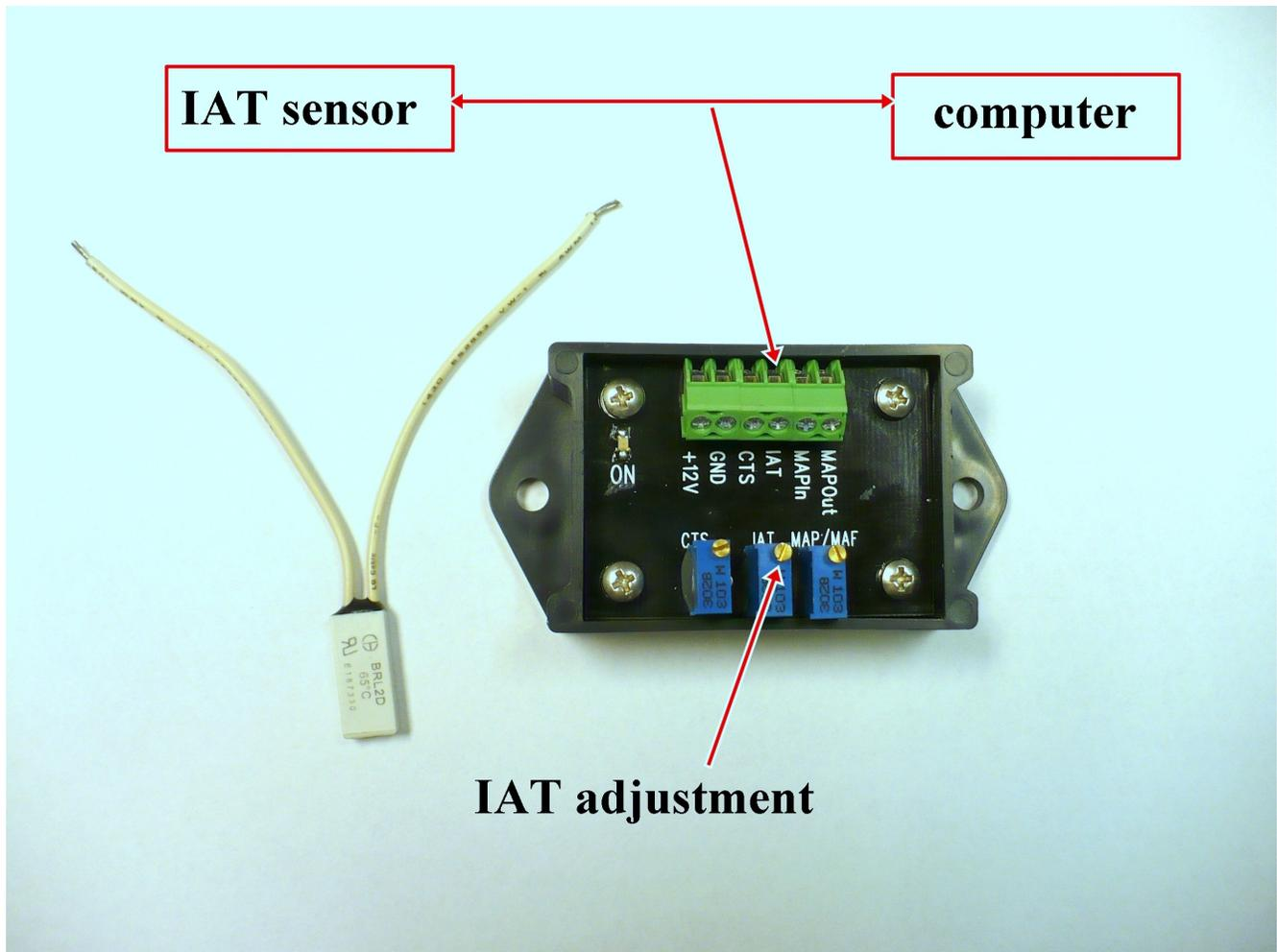
Locate your IAT ( intake air temperature ) sensor. There will be 2 wires going to the sensor. You will **NOT** be cutting any wires. You will skin off some of the insulation from the signal wire. Refer to your manuals diagram. Or you can refer to the document Identifying your signal wires. Solder on a length of wire sufficient in length to reach your AFR Control Center and attach it in the terminal marked IAT as pictured above.
