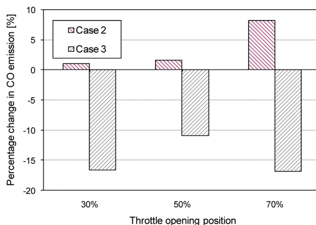
Figure 9. Average percent increase of CO emission relative to case 1 over the considered engine speeds
