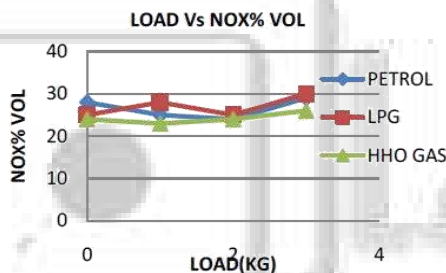
Fig. 4: variation of Nox Against with different load [3]
