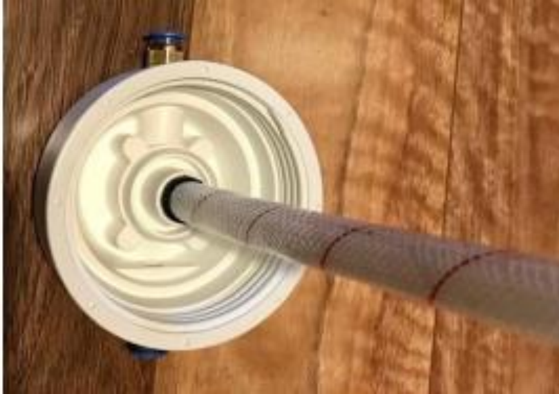
Fig. Bubbler assembly. Installers can create their own bubbler assembly based on the need of the vehicle. If not transparent plastic, it should be Stainless steel body with a visibility of water level inside the bubbler.
