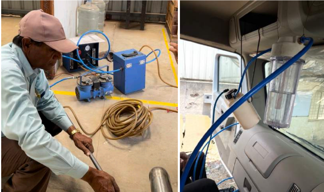
Figure 5. Emission testing equipment in operation
