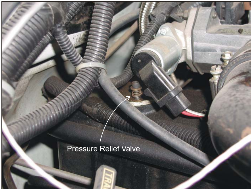
Figure 3-7 Pressure Relief Valve on Engine Crankcase
