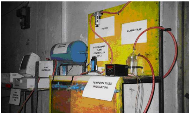
Fig. 4. Photographic view of the hydrogen flow arrangement.
