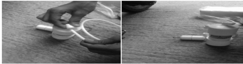
Figure 4: Hose Pipe to Booster Filled with Diluted Solution of Electrolyte
