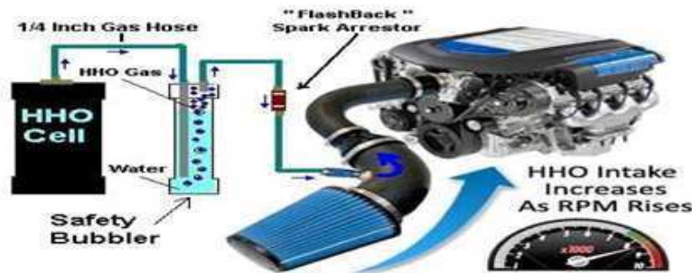
Figure 2: Hydrogen Intake in IC Engine with HHO
