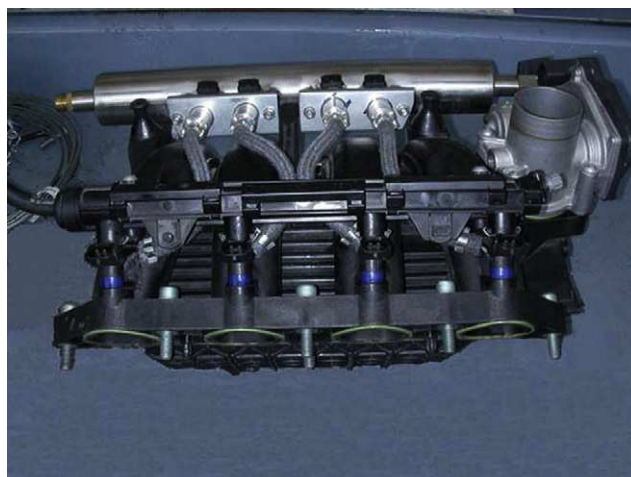
Fig. 2 – Intake manifold with the bi-fuel (hydrogen/gasoline) injection systems.
