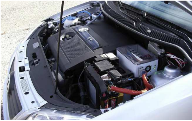
Fig. 6 – New MoTeC M400 programmable electronic control unit (bottom) connected to the electrical junction box.
