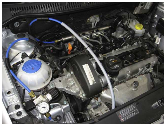
Fig. 3 – Bi-fuel intake manifold assembled in the engine compartment.
