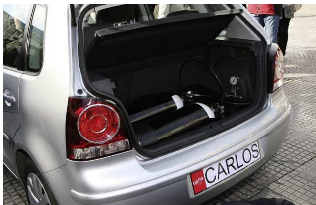
Fig. 4 – Gas cylinders for hydrogen storage at 200 bar placed in the car boot.
