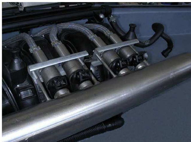
Fig. 1 – Hydrogen accumulator with the four hydrogen injectors.
