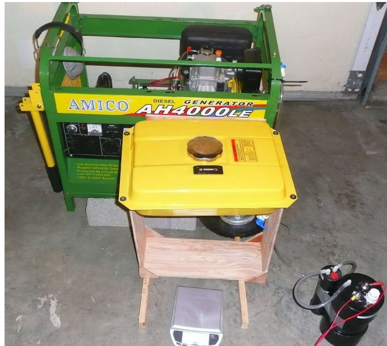
Figure 2: Generator/weight measurement set up
